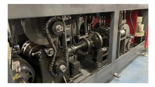
1. The whole Automatic intelligent paper cup machine adopts automatic oil lubrication system( oil circulation system is including oil motor, filter, copper pipe) which makes all gear moving parts working at high speed much more smoothly and greatly Improve the
