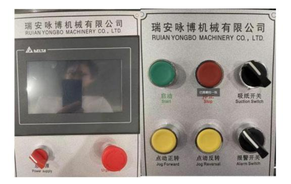
1,This **Automatic intelligent paper cup machine** Setting the rated speed is 55 times/min,is the fastest speed in china,it have the material control,sending paper control,molding control,Collection control etc. automatic system,if the machine conks out,it will be stoped and sounds the alarm
